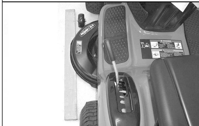
3. Place a straight 2x4 piece of wood (A) or a 38 mm (1.5 in.) thick block under the edge (B) of each side of mower deck.
