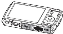
2. Unlock and open the battery/memory card compartment at the bottom of the camera.
