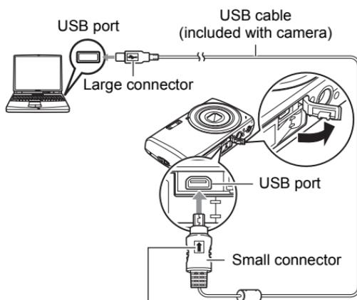
Making sure that the ↑ mark on the USB cable connector is towards the lens side, connect the cable to the camera.
