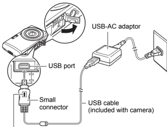
Making sure that the ↑ mark on the USB cable connector is towards the lens side, connect the cable to the camera.
