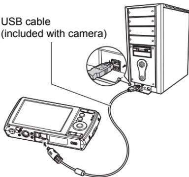
4. The USB mode menu appears on the screen. Select **Computer** by using the ▲ or ▼ keys and press the **OK** button.
