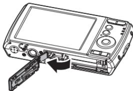
3. Insert the battery into the compartment with the terminal facing inside the camera with correct orientation as shown.
