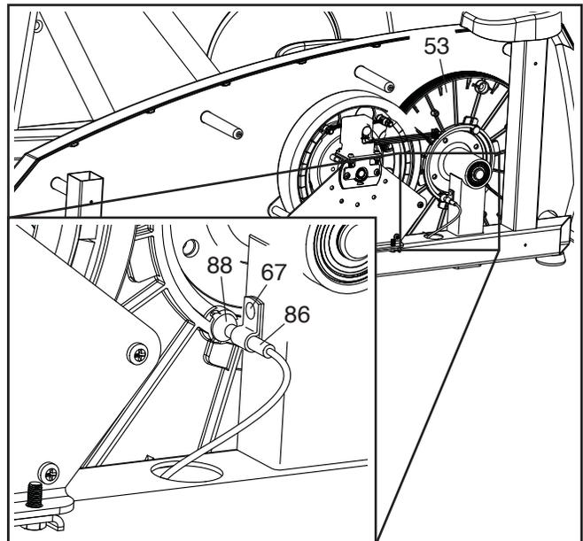
Loosen, but do not remove, the indicated M4 x 16mm Screw (67). Slide the Reed Switch (86) slightly closer to or away from the Magnet (88), and then retighten the Screw. Then, rock the Pulley (53) forward and backward just enough that the Magnet passes the Reed Switch repeatedly.
