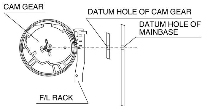
Fig.3-13 ASSEMBLY OF THE CAM GEAR & F/L RACK
