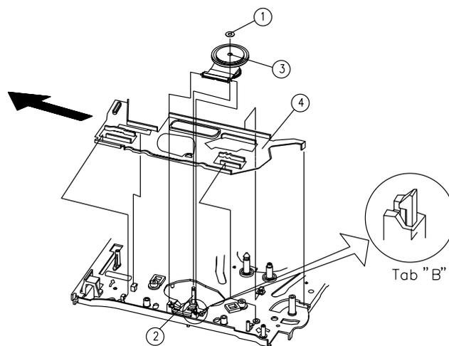
Fig.3-21 REEL GEAR TOTAL ASS'Y & CONNECT PLATE REMOVAL
