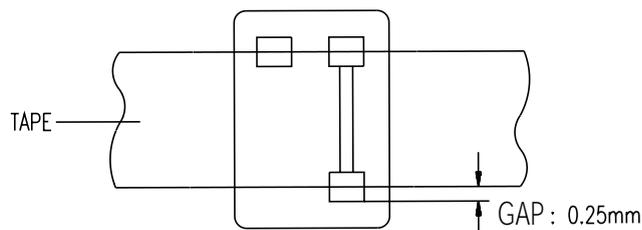
Fig. 5-4 A/C HEAD ASS'Y ADJUSTMENT (HEIGHT ADJUSTMENT)
