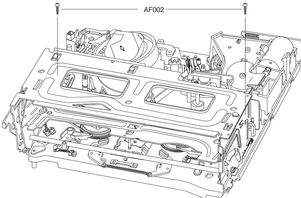
Fig.3-1 FRONT LOADING ASS'Y SEPARATION
