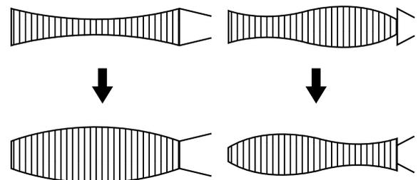
Fig.5-9 FINE TUNING OF THE ENVELOPE AT THE DRUM ENTRANCE/EXIT (II)
