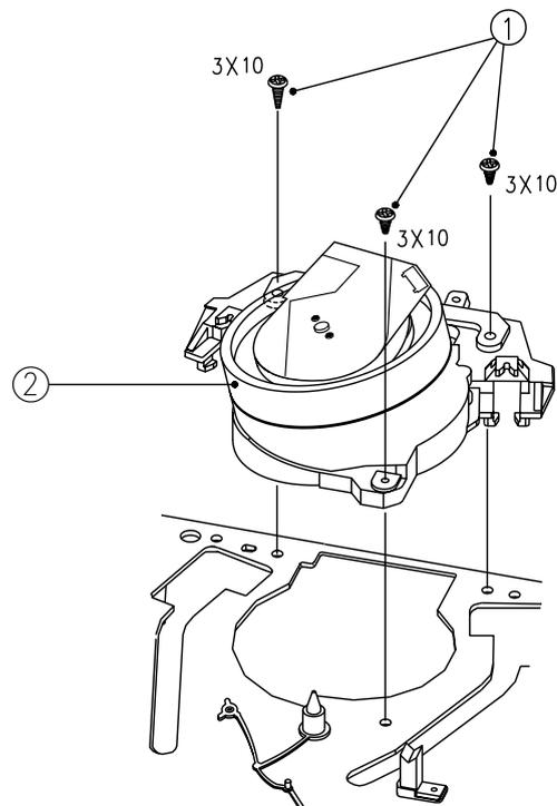
Fig.3-7 DRUM TOTAL ASS'Y & EARTH BRKT ASS'Y REMOVAL
