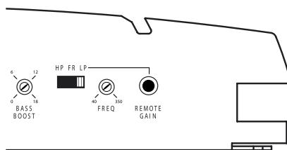
Note: If you are using the Remote Gain, make sure to take this into account during set-up procedures of the subwoofer amplifier. You should set the system up with the Remote Gain plugged in and with the level knob turned all the way down (counter-clockwise). The Remote Gain only works when you've selected the LPF (low-pass) crossover configuration.
