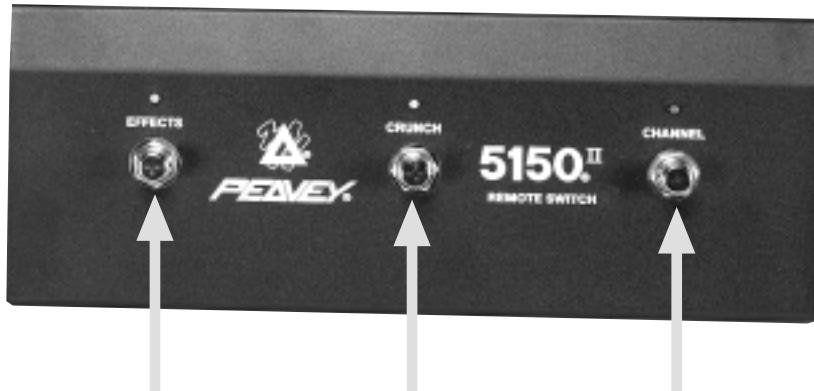
Activates Effects Loop when switch is pressed and LED illuminates
