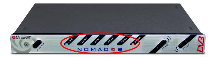
**LNB:** When lit, this LED indicates the coax cable from the receiver has been correctly connected to the NOMAD 2 Universal Controller, and the receiver has power. (**Note:** The LNB LED is illuminated once the coax cable of the receiver has been connected, but does **NOT** indicate the Controller has power).
