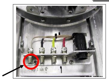
When using the HD-DP3 for a Dish Network system, this connection is used for "IN" only and <u>not used for</u> "OUT". Its use is for input from an external dish. Do not use this connection to input to the Nomad 2 or input to a satellite receiver.
