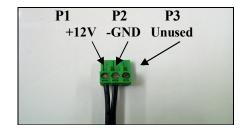
**Power Connector:** Is used to connect the 12 VDC <u>4 AMP</u> power supply to provide power to the NOMAD 2 Universal Controller. (<u>Note</u>: Only use the power supply provided by MotoSAT.)
