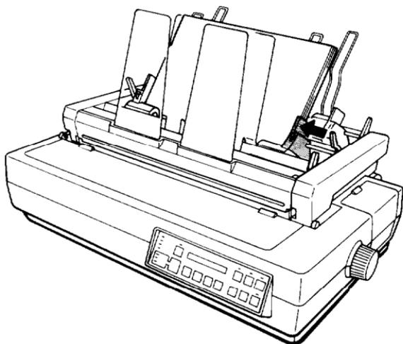
5. Push the paper levers back until the paper is clamped against the guide rollers. The levers will not close completely if too much paper is used. If this happens, remove some paper from the stack and try again.
