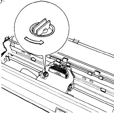
7. Slide the print head from side to side to make sure **that** it moves smoothly. (Do not try to slide the print head by grasping the ribbon cartridge.)
