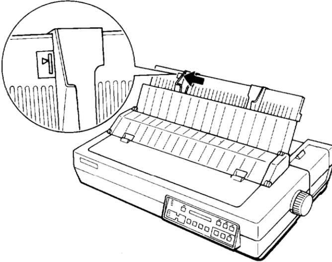
4. Adjust the right edge guide to match the width of your paper. Next, slide a sheet down between the edge guides until it meets resistance.
