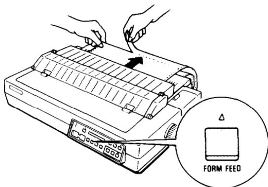
**Note:** If the perforation of **the** paper is not fed past **the edge** of **the** paper guide **the** first time, press **the FORM FEED** button again. Do not use **the** platen knob to feed the paper.
