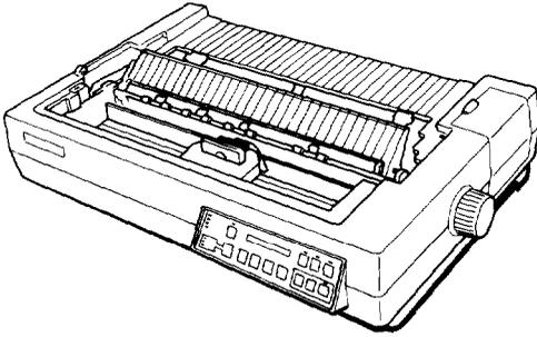
2. Remove the paper eject guide by tilting it forward, then lifting it up and off.
