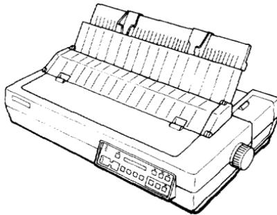
1. Be sure that **the** printer is off line. If it is **not**, press the **ON LINE** button to set the printer off line.
