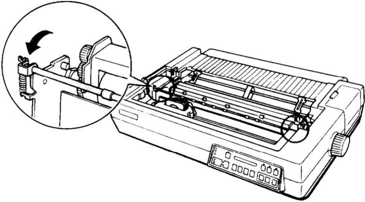
4. Hold the assembled cut sheet feeder in both hands and fit its notches over the red pins in the printer.
