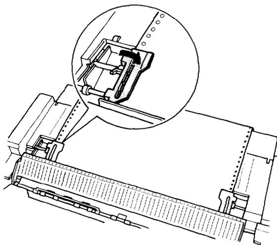
7. Slide the right sprocket unit to a position where the paper is straight and has no wrinkles, and then lock it into place.
