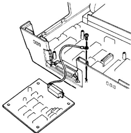
2. Holding the interface board level, rotate it clockwise into position and **attach** it to the main board. Make sure the connector pins are properly inserted into the mating connector.
