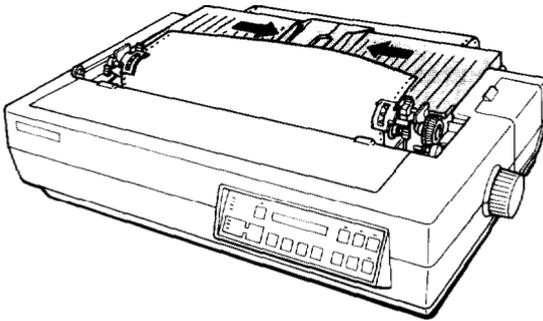
11. **Align** the pins of the pull tractor cover with the slots on the printer and attach the cover.
