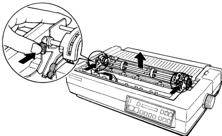
2. Replace the paper eject guide by fitting its notches onto the pins inside of the printer at each side, then tilting the guide back slightly.
