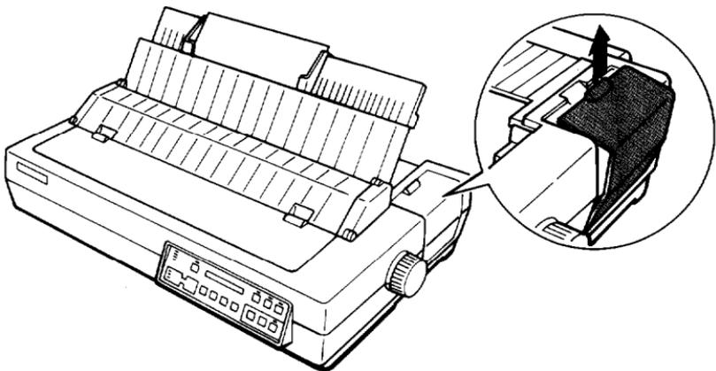
2. Plug the Multi-Font Module carefully into either Slot A or B. The arrow on the module should point toward the printer.
