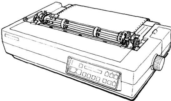
3. After the paper is loaded in the push tractor, see that the printer is off line. Press the **LOAD/EJECT** button to load the paper. Then press the **FORM FEED** button to advance the paper one page so that you can fit the paper onto the pull tractor.
