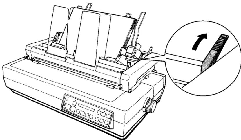
6. You can choose to have the printer eject the sheets with the printed side facing downward or upward. To have the printer eject the sheets with the printed side facing downward, pull the front lever on the right side of the cut sheet feeder forward. To eject the sheets with the printed side facing upward, push this lever back.
