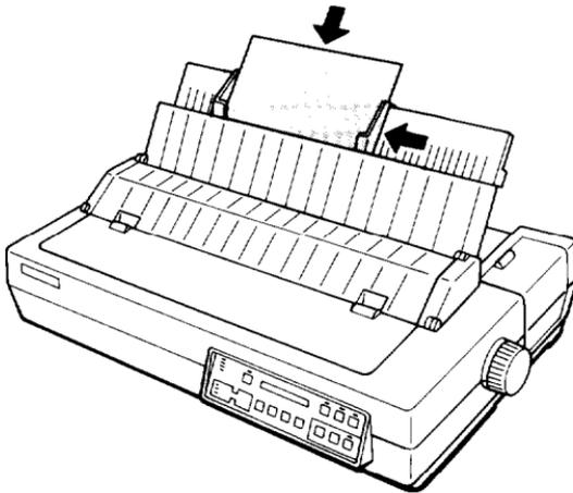
Run the self test using paper wider than A4 size (8.27 inches).
