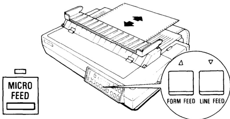
Note: The printer beeps when the paper reaches a position that is approximately 1/3 of an inch from the top edge of the paper. You can use this position as a reference point when you adjust the printer's loading position.
