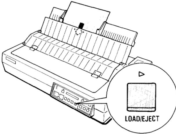
Note: If the platen turns without loading the paper, completely remove **the** paper and re-insert it more firmly; then press the **LOAD/EJECT** button again.
