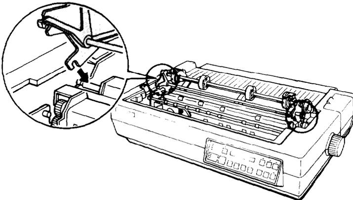
5. Tilt **the** tractor unit toward you until the front latches click in place over the red front mounting rods of the printer.
