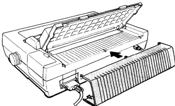
Note: The cable cover should always be attached when you use the printer.
