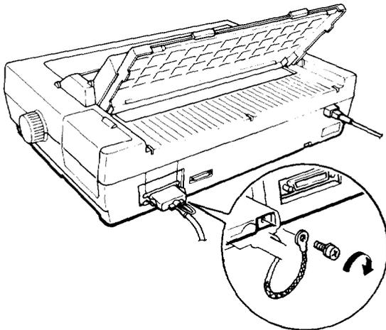
4. Plug the other end of the cable into the computer. (If there is a ground wire at the computer end of the cable, attach it to the ground connector of the computer.)
