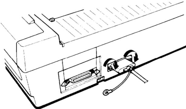
**Note:** If the screws that come with the cable do not fit into the connector lock nuts on the interface, you need to replace these lock nuts with the optional lock nuts provided with the printer.
