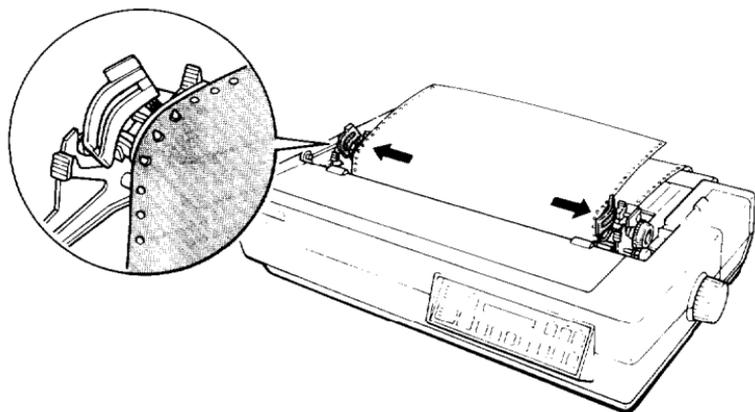
7. If the paper does not fit exactly onto the tractor pins, press in on the pull tractor feed knob and turn it in the desired direction.
