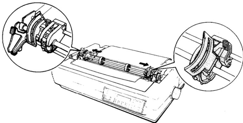
6. Fit the holes of the paper over the tractor pins of the sprocket units, adjusting the position of the sprocket units as necessary.
