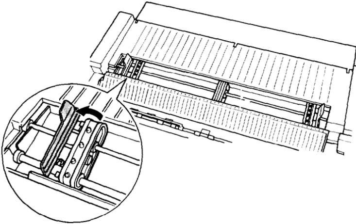
5. Fit the first four holes in the continuous paper over the pins of the sprocket units.
