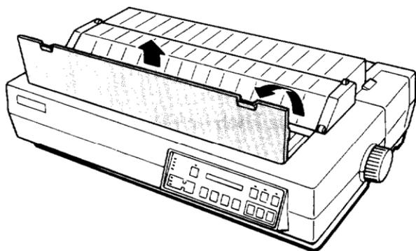
2. Open the paper guide cover as shown in the illustration. Then raise the rear of the cover slightly and lift the cover away from the printer at a slight upward angle.
