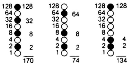
With this numbering system, every combination of the eight pins adds up to a decimal number between 0 and **255**, and no numbers are duplicated.
