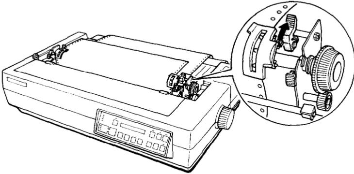
10. Attach the paper guide and lower it so that it is resting on top of the printer. Center both edge guides.
