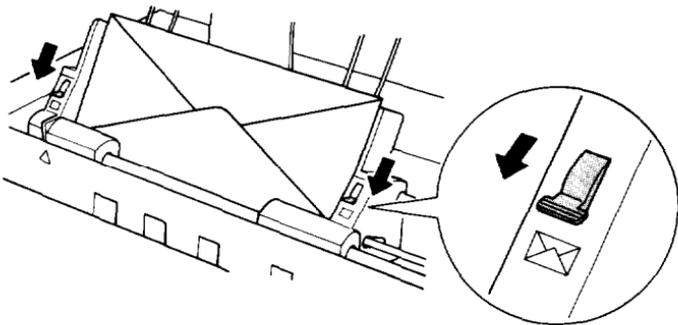
3. Press the **LOAD/EJECT** button to load an envelope. Then press the **ON LINE** button to start printing.
