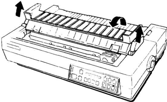
3. Remove the print head protector and white foam packing material.
