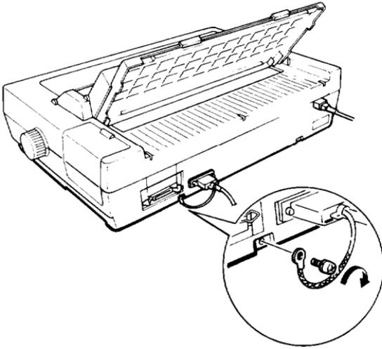
4. Plug the other end of the cable into the computer. (If there is a ground wire at the computer end of the cable, attach it to **the** ground connector of the computer.)
