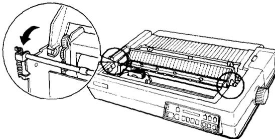
3. Remove the paper eject guide by tilting it forward, then lifting it up and off.
