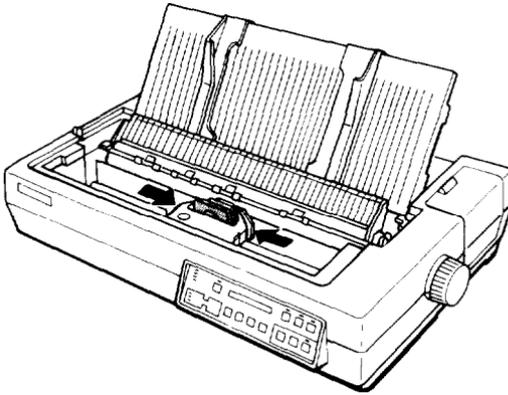
3. To release the ribbon cartridge, gently press the tab at the top of the holder; then lift the cartridge straight up and out of the printer.
