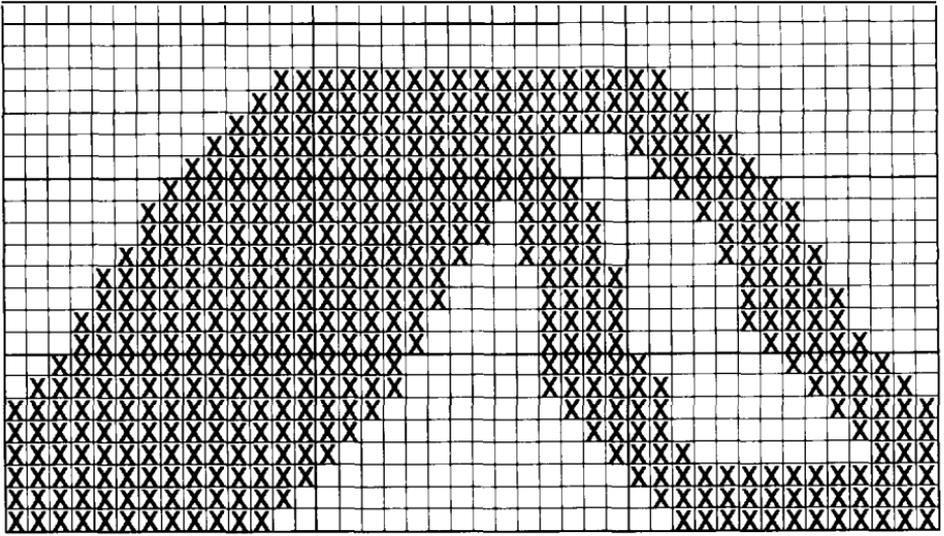
The actual pattern **that** the printer prints on **the** paper is made up of dots that overlap each other both vertically and horizontally. The reason the planning grid uses **an x** for **each** dot is that using an accurate representation of **the** dots makes calculating the data numbers difficult because they cover each other. Therefore, remember that **each x** represents the center of a dot, and the dots actually overlap.
