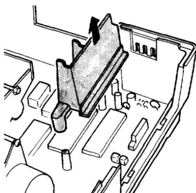
7. Remove the shield plate above the parallel interface by pressing in on the plastic clips located at the back of the plate. (The following illustrations show a rear view of the printer.)
