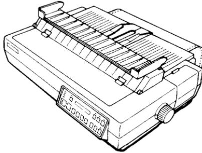
1. Press the **PAPER SELECT** button until the **FRICTION** light comes on. The continuous paper is fed backward automatically to a standby position.
