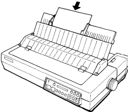
5. Press the **LOAD/EJECT** button once to automatically load the paper.
