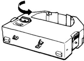
5. Hold the ribbon cartridge while gently squeezing the two ridged plastic tabs together; then lower it until it snaps into place. The side hooks in the printer should fit into the slots on each side of the ribbon cartridge.
