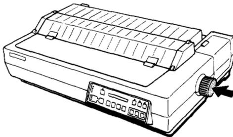
**Caution:** Using the platen knob to adjust the position of the paper interferes with the automatic paper loading system and may cause a paper **jam**. If you need to adjust the position of the paper after it is loaded, use the micro-adjustment feature described in the section on setting the loading position in Chapter 3.
