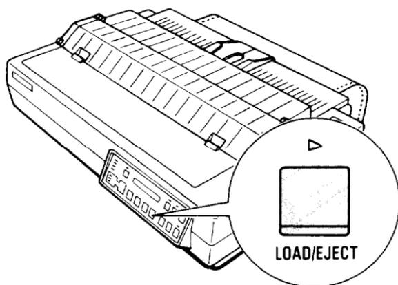
**Note:** If you press **the** **LOAD/EJECT** button when continuous paper is already loaded, **the** paper is reversed to the standby position.
