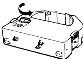
5. Hold the ribbon cartridge while gently squeezing the two ridged plastic tabs together; then lower it until it snaps into place. The side hooks in the printer should fit into the slots on each side of the ribbon cartridge.
