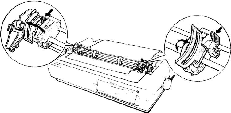
5. Adjust the sprocket units to match the width of the paper and adjust the paper supports so they are evenly placed between the sprocket units.
