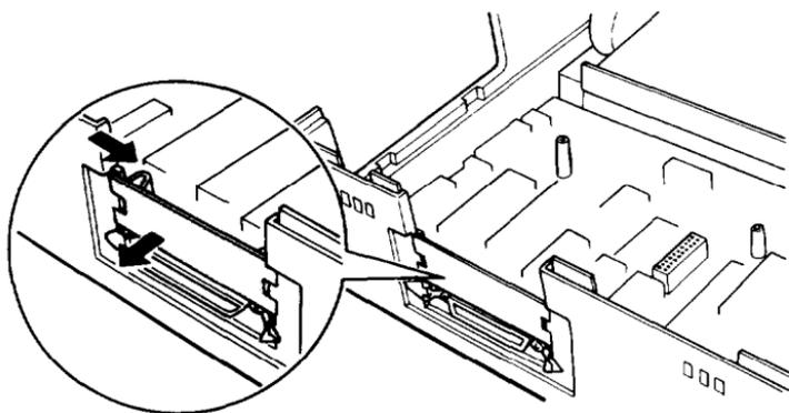
8. Remove one of the screws labelled CG (chassis ground) from the main board. The illustration shows you the location of the CG screw that you should remove.
