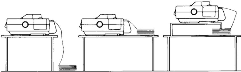
Be sure to align your paper supply with the paper loaded in the tractor so that the paper feeds smoothly into the printer.
