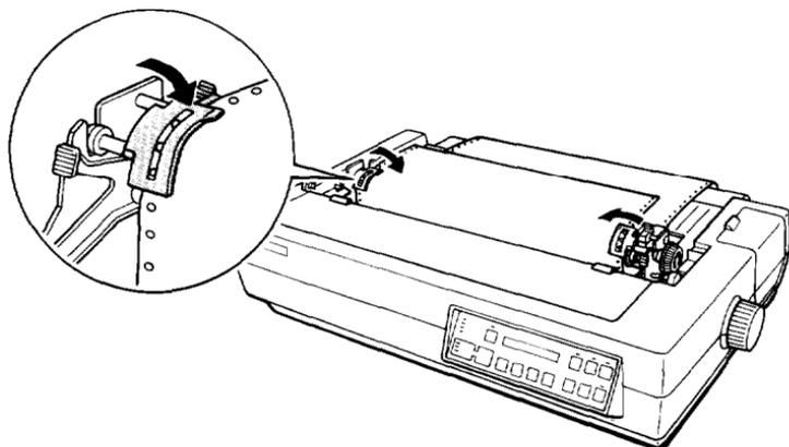
9. See that the paper is not crooked or wrinkled and lock the sprocket units in place.
