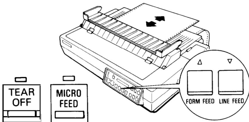
**Caution:** The short tear-off feature can only be used with the built-in tractor feeding system.
