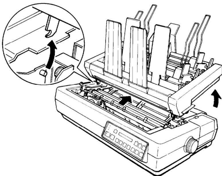
2. Replace the paper eject guide by fitting its notches onto the red pins inside the printer at each side, then tilting the paper eject guide back slightly.
