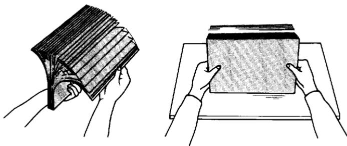
4. Insert the paper along the left paper guide. Then, adjust the position of the right paper guide so that it closely matches your paper's width. Be sure that the position of the guide allows the paper to move up and down freely.
