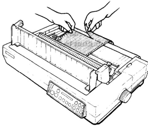
4. Press the **ON LINE** button to set the printer off line. Then press the **FORM FEED** button to eject the labels. (Remember not to use the **LOAD/EJECT** button to eject labels.)
