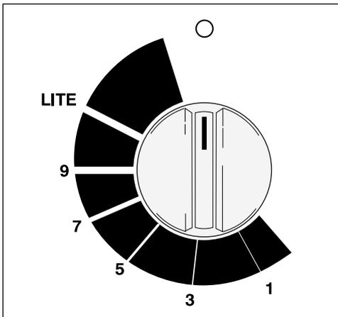
Each burner lights automatically from an electric ignitor each time a control knob is turned to the LITE position. Two ignitors (one per set of burners) are supplied.
