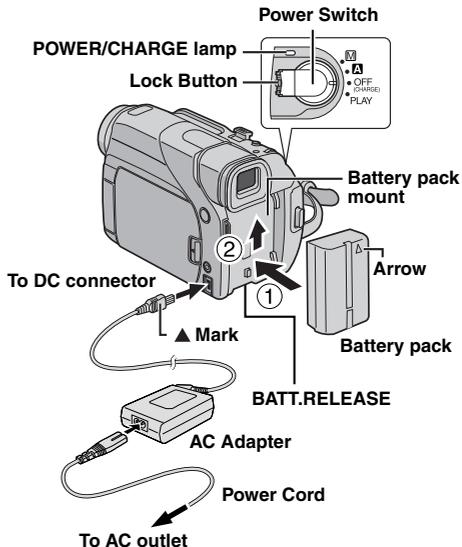
This camcorder's 2-way power supply system lets you choose the most appropriate source of power. Do not use provided power supply units with other equipment.
