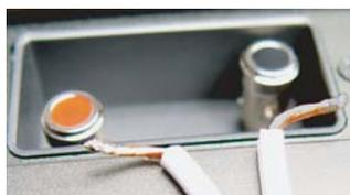
Always be careful to observe proper polarity, making sure to connect (+) to (+) and connect (-) to (-). Failure to do so will cause a loss of low frequency response and improper imaging.
