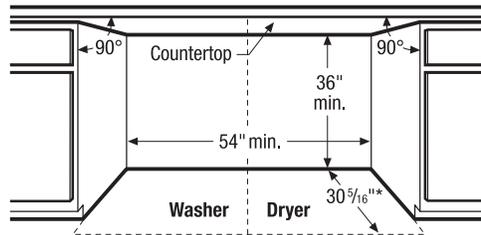
**Side-by-Side Units in Under-Counter Installation**
