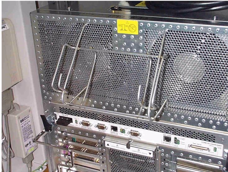
2. Place the Secure Web Console power supply into the bottom portion of the wire mounting bracket as shown.
