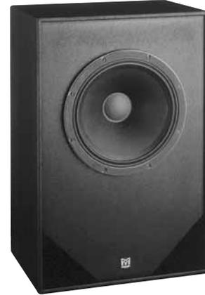
Screen Sub 1A provides low distortion, true sub-bass response for any cinema environment. Built with a shallow profile, like the Screen 4 and Screen 5, the sub is designed for behind-the-screen placement. The unit uses a single 18" (460mm) long excursion high power driver. Large area tapered twin ports ensure minimum turbulence down to the lowest frequencies demanded by today's digital sound tracks.
