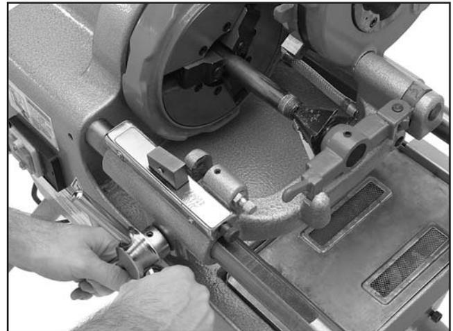
**Figure 12.** Typical reaming operation.
