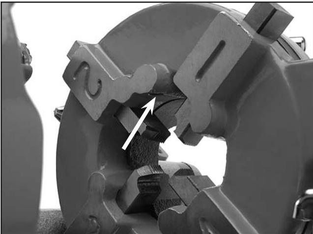
**Figure 24.** Fluid flow location with threading tool down.
