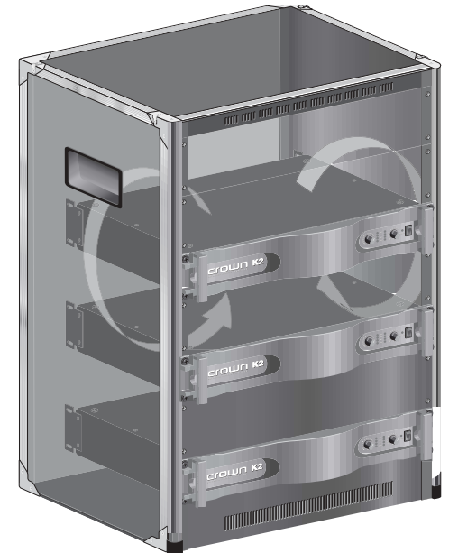
Figure 3.2 Spacing the Amplifiers in the Rack Improves Cooling
