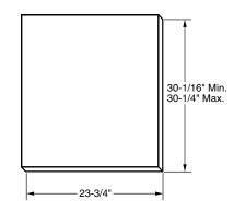
• The top of the custom panel must be flush with the top of the door. The 1/2" minimum gap between the top of the door and the bottom of the countertop must be maintained.
