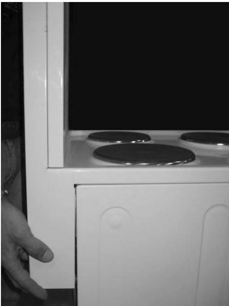
5. Fix the Grill assembly to the cooker using three screws on the right-hand side and three screws on the left-hand side as shown in the photograph, using the screws supplied.
