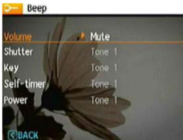
3. Press the Right button, press the Up/Down button to adjust volume and change tone, and press the
