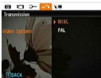
The video output signal can be switched to NTSC or PAL to accommodate different regional standards. The appropriate setting will vary between regions.
