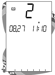
Fig. 72 - Log Mode (during Transition Period)
