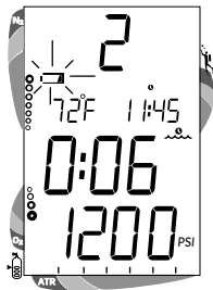
Fig. 9 - Low Battery Condition
