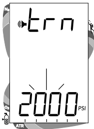
Fig. 34 - Set Turn Pressure Alarm
