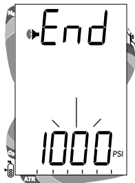
Fig. 35 - Set End Pressure Alarm
