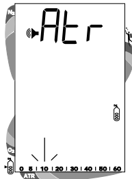
Fig. 33 - Set Air Time Remaining Bar Graph Alarm
