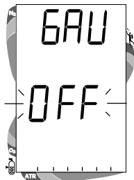
Fig. 41 - Set Digital Gauge Mode
