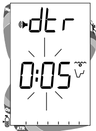
Fig. 36 - Set Dive Time Remaining Alarm
