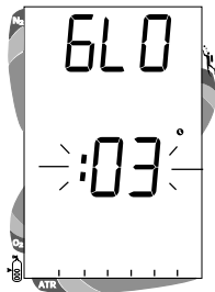
Fig. 39 - Set Backlight Duration
