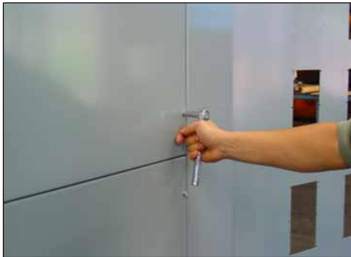
Figure 39. Removing the Bolts.
