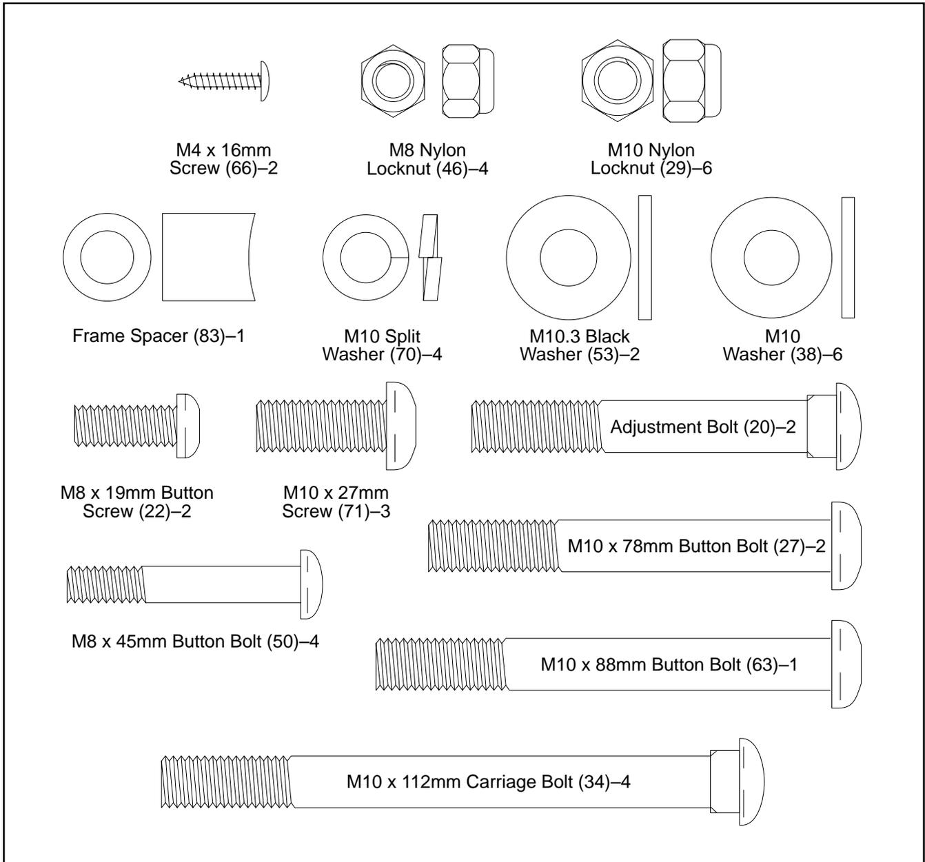
1. Identify the Front Stabilizer (3), which has Wheels (32) attached to it. While another person lifts the front of the Frame (1), attach the Front Stabilizer to the Frame with two M10 x 112mm Carriage Bolts (34) and two M10 Nylon Locknuts (29). **Make sure that the Front Stabilizer is turned so the Wheels are not touching the floor.**
