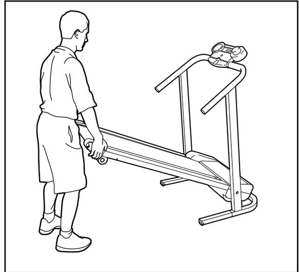
2. Move your right hand to the position shown and hold the treadmill firmly. Raise the treadmill until the latch pin is aligned with the hole in the left upright. Slide the latch pin into the hole. **Make sure that the latch pin is inserted as far as possible into the hole.** Lock the pin by pressing the end of the pin into the slot in the storage latch as shown in the inset drawing.
