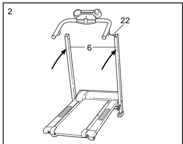
3. Push the Wire Harness (22) into the right Upright (6) as you insert the Handrail (16) into the right and left Uprights (6). **Be careful not to pinch the Wire Harness.** Tighten a Handrail Bolt (12) with a Washer (11) into each Upright.
