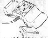
Insert 4 Alkaline "AAA " batteries, UM-4, LRO3 or equivalent into the battery compartment. Close the compartment.
