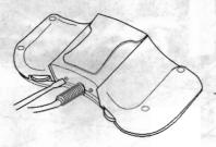
Unscrew the screws which are on the battery cover in the bottom part of the control pad.
