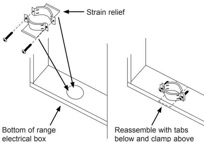
5. Slide the end of the appliance cord into the strain relief from the bottom of the box. See facing page.
