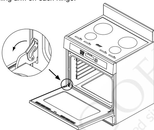
3. Lift the oven door to about a 15° angle from the vertical position.
