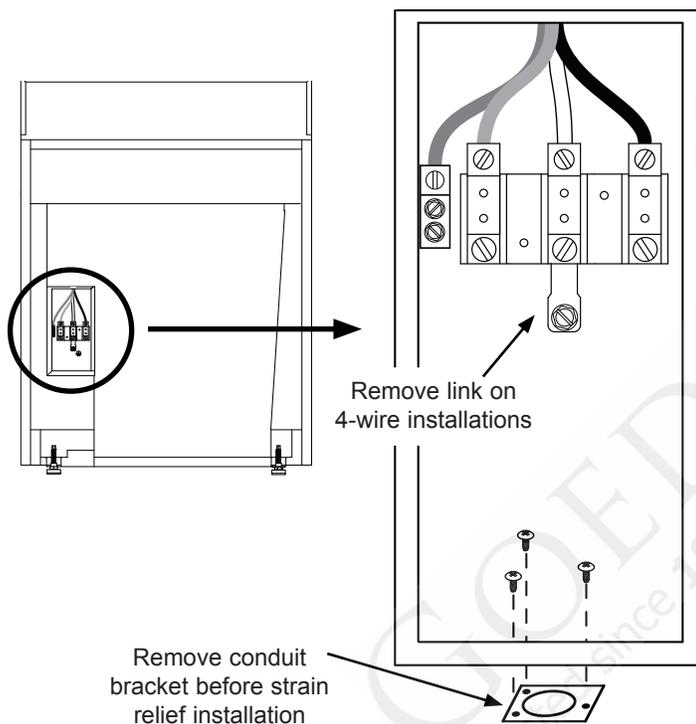
4. Disassemble and remove the strain relief from the appliance cord (not included). Insert the tabs on the two parts of the strain relief into the hole on the bottom of the box and reassemble it so that the tabs are below the box and the strain relief itself is inside the box.
