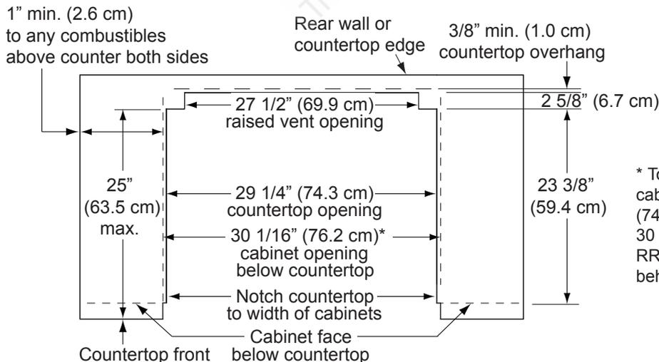
\* To create a “built-in look” on the front of the cabinet, this dimension may be changed to 29 1/4” (74.3 cm), with the width at the notches remaining 30 1/16”. This configuration is only for models RR30NIS and RR30NIFS with the side panels behind the door removed.
