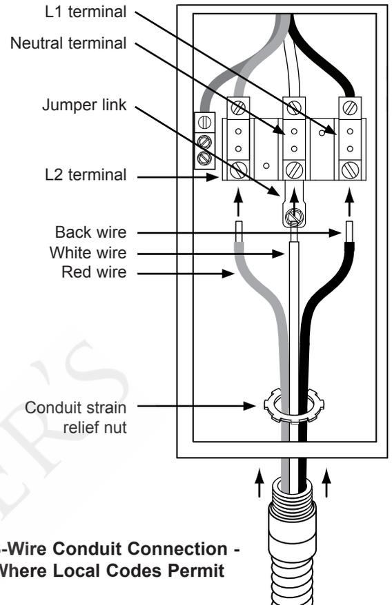
5. Before connecting the wires, slide the strain relief nut over the wires and thread it onto the conduit strain relief inside the box. Tighten into place.
