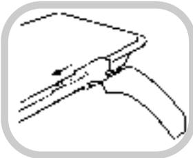
Slide the handle towards the centre of the pan and let the handle locate over the bracket.
