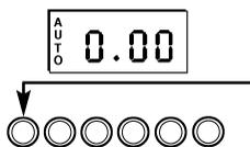
**Note 1** When the Minute Minder has been set, the time remaining can be checked at any time by simply pressing the Minute Minder button.
