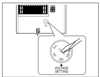
Use a screw driver to rotate the voltage selector so the voltage number the voltage mark is pointing at is the same as the voltage where you are plugging the this unit. (See the back cover page.)
