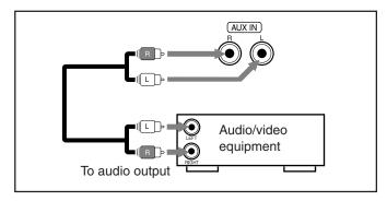
For playing the other equipment through this unit, connect between the audio output jacks on the other equipment and AUX IN jacks by using audio cords (not supplied).
