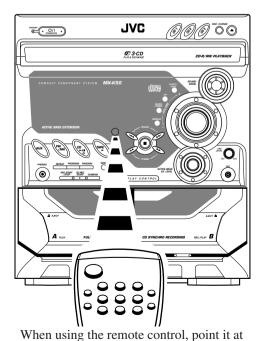
the remote sensor on the front panel.
