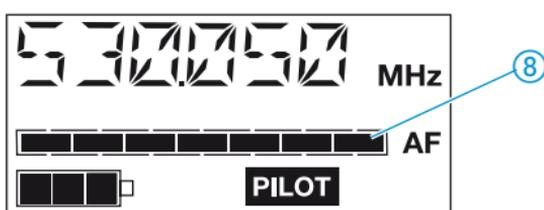
If, on the other hand, the sensitivity is adjusted too low, the transmission link will be undermodulated, which would result in a signal with high background noise.
