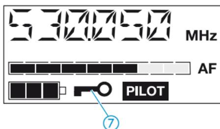
To deactivate the lock mode, first press the **SET** button and then press the **▲/▼** buttons to select “**LOC.OFF**”. If you confirm your selection by pressing the **SET** button, the buttons can be operated as usual.
