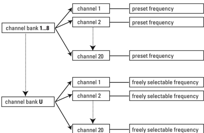
Each of the channels in the channel banks "1" to "8" has been factory-preset to a transmission frequency (see enclosed frequency table). These transmission frequencies cannot be changed but have been preset so that e.g. country-specific regulations on frequency usage are taken into account.
