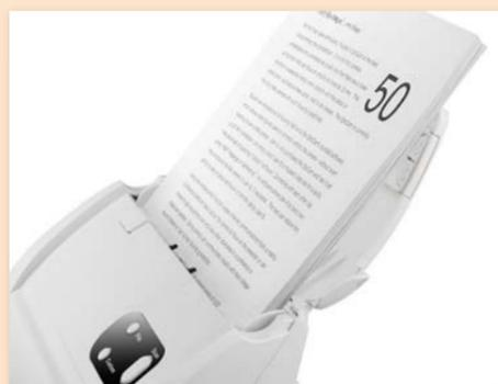
A redesigned 50 page Automatic Document Feeder with a 3000 page per day duty enable the SmartOffice PS340S to be used in any application requiring frequent document and rigid card scanning.
