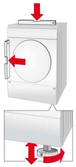
The dryer should be level with all feet firmly on the ground. The dryer must not wobble.
