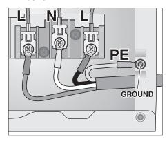
The appliance is now ready to be plugged into the 4-wire receptacle of the power rating.
