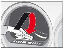
This deposit can easily be removed by wiping the sensors (the two bars next to the lint filter) with a cloth and a little white vinegar.
