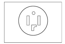
When installing the receptacle for the dryer cord, ensure that the power supply cord is accessible when the dryer is in the installed position.
