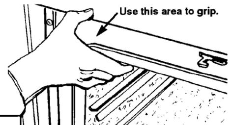
**6.** Remove and discard shipping base or cardboard or hardboard from under range. Lift range up to cabinet opening using the oven opening as an area to grip.
