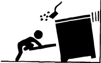
To reduce the risk of tipping the appliance, the appliance must be securely fastened to the cabinet using the four screws that are provided.
