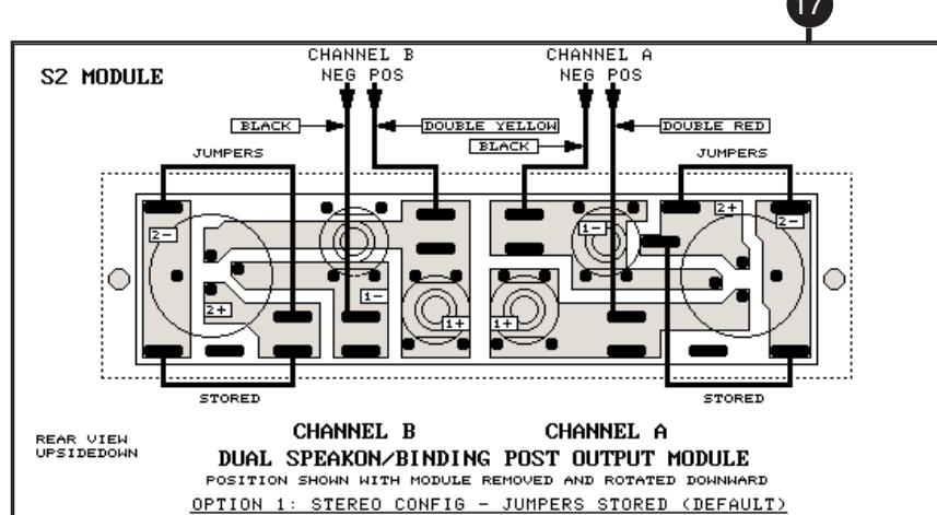
**WARNING:** The S2 module is shipped with four jumpers plugged in a “storage” configuration across the normally unused 2+ and 2- Speakon pins. These jumpers are used in other modes of operation following. This “storage” configuration could cause a shorting problem if a particular loudspeaker system’s Speakon connectors are wired in the high current configuration outlined next (1+ and 2+ are connected and 1- and 2- are connected). In this case, we recommend that you remove the jumpers.
