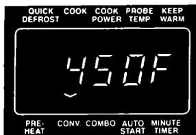
When the oven temperature reaches 450°F, the oven beeps twice and the PREHEAT Indicator Light goes off. "450F" will stay on the Display and the oven will hold that temperature up to 30 minutes, or until the food has been placed in the oven and START has been touched. **NOTE: The oven will automatically shut off and the Display will show the time of day if food has not been placed in the oven within 30 minutes.**
