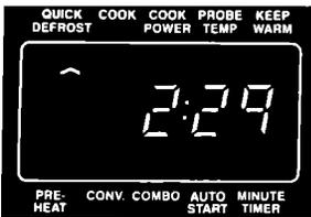
The QUICK DEFROST Indicator Light will stay on to show that the oven is in the Quick Defrost Cycle.
