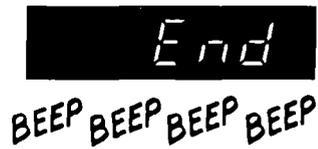
When the Cook cycle ends, "End" will show on the Display and 4 beeps will sound. (You can stop the beeping by opening the door or by touching CANCEL.) "End" will remain on the Display and a beep will sound every 60 seconds (to remind you that food is left in the oven) until the door is opened or CANCEL is touched. The Display will then show the time of day.
