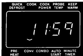
The Display will count down the cooking time to show how much time is left in the broiling cycle.
