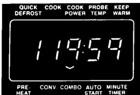
The COMBO Indicator Light will come on and the Display will count down the cooking time to show how much time is left in the cooking cycle.
