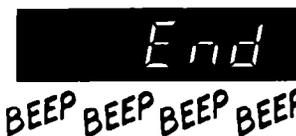
When the Broil Time cycle ends, "End" will show on the Display and 4 beeps will sound. (You can stop the beeping by opening the door or by touching CANCEL.) "End" will remain on the Display and a beep will sound every 60 seconds (to remind you that food is left in the oven) until the door is opened or CANCEL is touched. The display will then show the time of day. The fan will continue to run until internal oven parts have started to cool.
