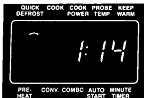
The QUICK DEFROST Indicator Light stays on and the Display counts down the remaining time.
