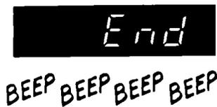
When the Roast Time/Combo cycle ends, "End" will show on the Display and 4 beeps will sound. (You can stop the beeping by opening the door or by touching CANCEL.) "End" will remain on the Display and a beep will sound every 60 seconds (to remind you that food is left in the oven) until the door is opened or CANCEL is touched. The display will then show the time of day. The fan will continue to run until internal oven parts have started to cool.
