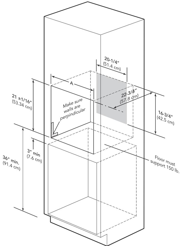
**Note:** Electrical outlet should not be located in shaded area.
