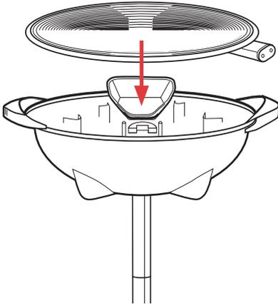
7. Position probe receptacle through probe cutout in top side of grill base.
