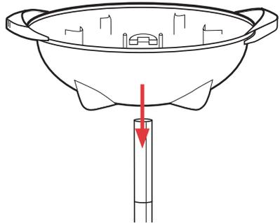
5. Place grease tray securely into position inside grill base. When properly placed, it is held firmly with pointed end in centre of grill base.
