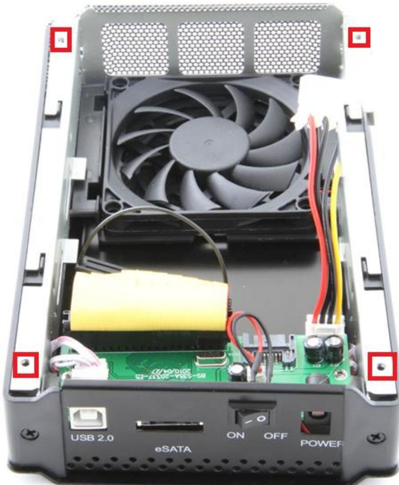
1. Locate the SATA data port on the enclosure. Plug one end of the SATA data cable into the port.
