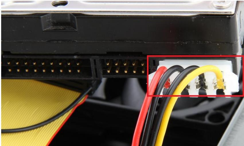
4. Locate the IDE data cable. Connect it to the IDE data port on your drive.
