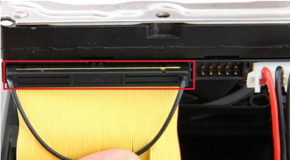
5. Insert the hard into the enclosure, as shown below:
