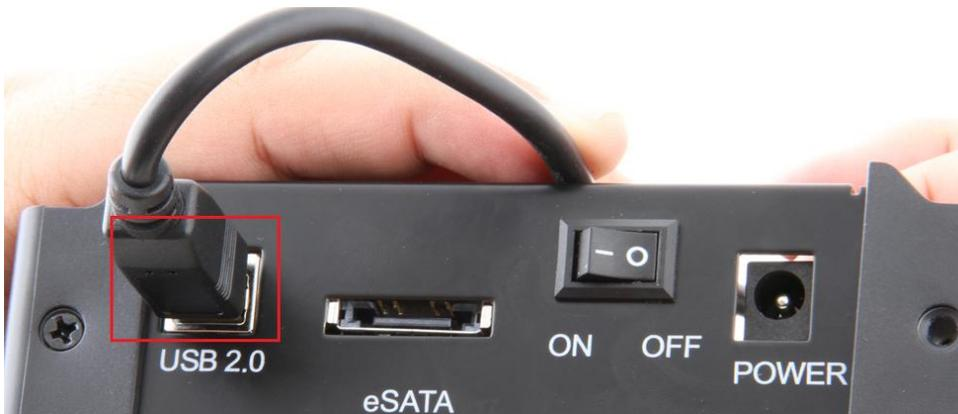
Alternatively, connect the E-Sata cable into the E-Sata port if you require it. (Note: E-Sata connector may be a bit difficult to plug in, and may require a bit of force to properly connect)
