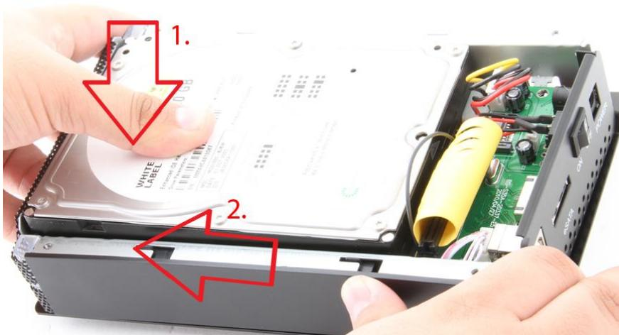
6. Place the **cover** back on the enclosure. **Screw** it back in place:
