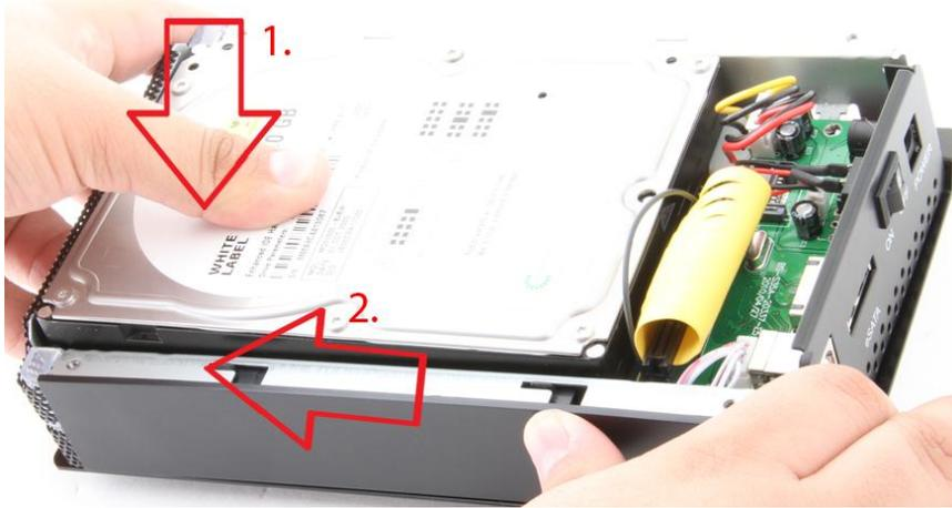
6. Place the **cover** back on the enclosure. **Screw** it back in place:
