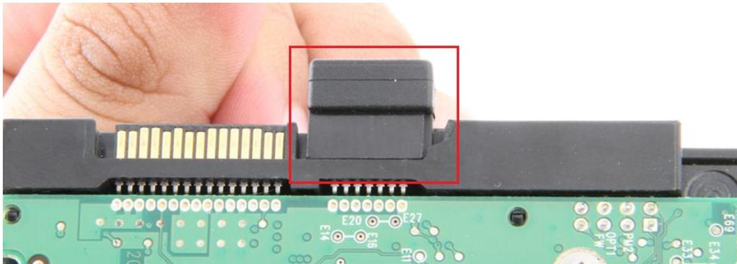
3. Remove the IDE power cable from the enclosure. Attach the SATA power cable in the same plug:
