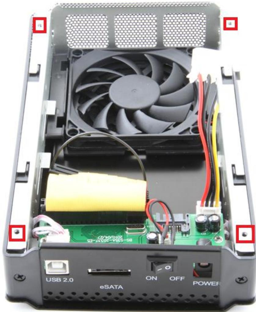
3. Locate the IDE power cable. Connect it to the IDE power port on your drive:
