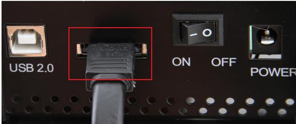
2. Connect the power cable into the power port on the enclosure.
