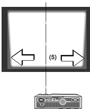
**3** Turn the focus ring and adjust the focus of the screen
