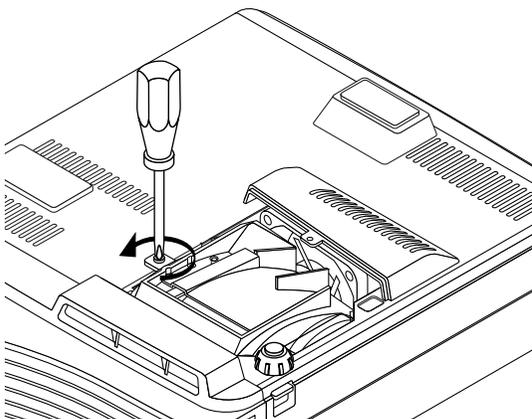
(2) Grasp the lamp cartridge's handle and pull upward to remove the lamp cartridge.
