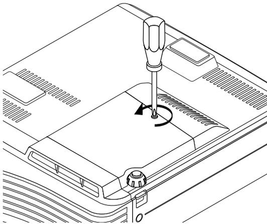
(2) Open the lamp cover a little, then pull it in the direction of the arrow and remove it.
