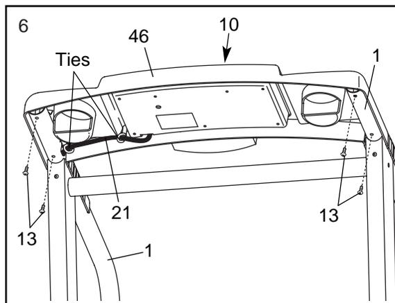
7. Attach the Console (10) to the Console Base (46) with seven 3/4" Screws (13). **Make sure that no wires are pinched.** Start all seven Screws before tightening them; **do not overtighten the Screws.** Note: Make sure the indicated 3/4" Screw is not overtightened. Overtightening the Screw may cause the Console to not function properly.
