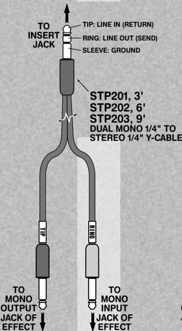
Connecting to the effect with a stereo-to-mono adapter and cables:
