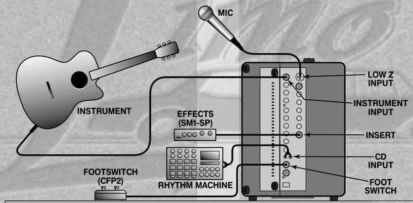
**Idea 2 – Play along:** Connect an instrument (acoustic or electric guitar, keyboard) to the Instrument Input jack. Connect a tape player or CD player to either the CD Input jacks or to the Low Z jack of the remaining channel. (See the notes on page 10 for more detailed information.) A pair of stereo headphones may be connected to the Headphones jack for privacy.
