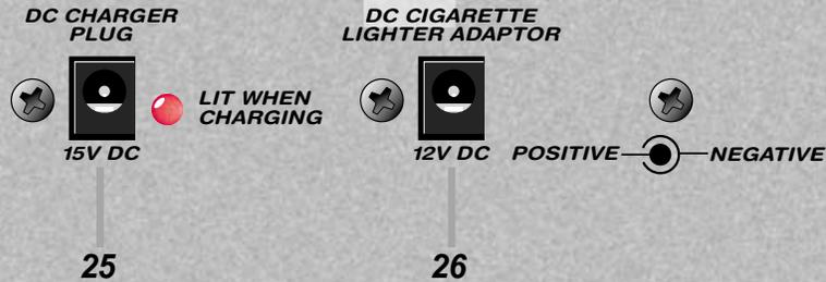
25. DC CHARGER PLUG, 15VDC: Plug the small round connector of the supplied AC wall adapter into this jack to charge the internal battery. The LED next to the jack glows red when the amp is charging. See page 4 for additional information.
