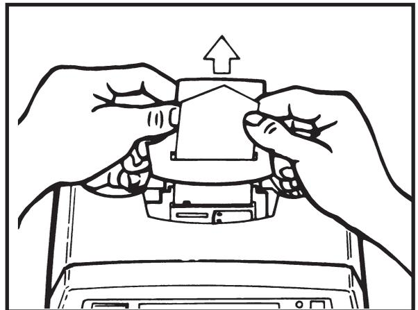
Figure 4 - Pulling printer paper through its cover
