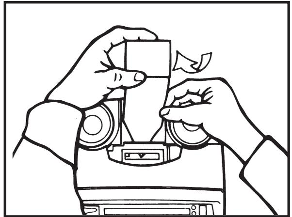
Figure 3 - Installing printer paper
