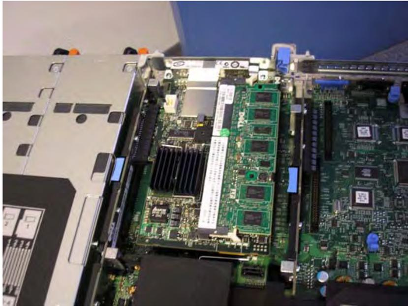
7. The next photo shows the Dell 2950 top cover off with PERC 5/E external RAID inserted.
