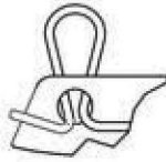
Figure 4-5. Create a loop from the power cable and feed it through the hole at the top front of the divider.
