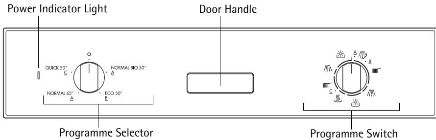
Set the point at which the wash programme is to start using the **programme switch**. The programme switch rotates during the wash programme and indicates the position that has been reached in the programme.
