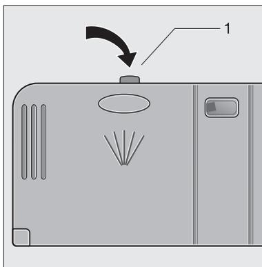
2. Fill the detergent dispenser with detergent. The markings indicate the dosing levels:
