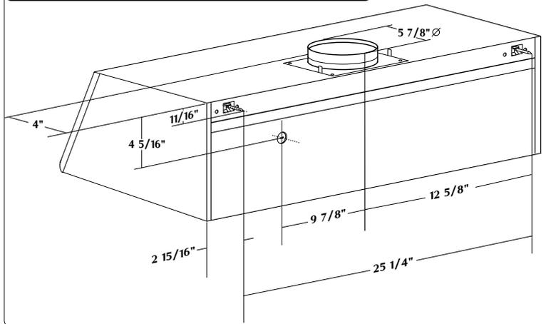
**FIG.02b Duct / Bracket / Electrical Dimensions 36" Hood**
