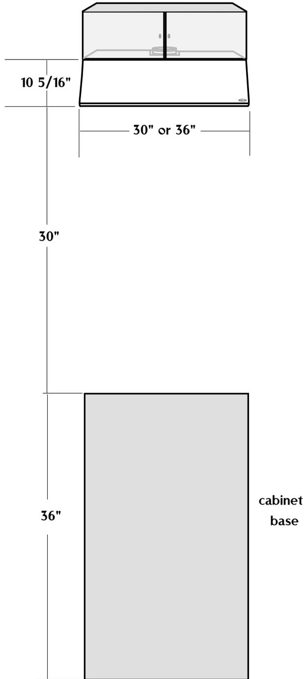
**FIG.05B CEILING HEIGHT VARIANCES WITH OPTIONAL CHIMNEY KIT (SIDE VIEW)**
