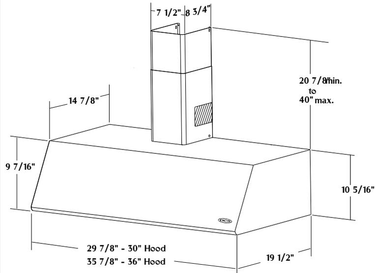
**FIG.02a Duct / Bracket / Electrical Dimensions 30" Hood**
