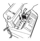
7 Pull the cartridge towards the front of the machine until you hear it click into position.
