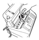
4 Remove the new cartridge from its packaging. Holding it by the finger grip, peel the protective film from the print nozzles.
