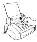
Remove the print cartridge from its packaging. Holding it by the finger grip, peel the protective film from the print nozzles.
