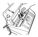
4 Remove the new cartridge from its packaging. Holding it by the finger grip, peel off the protective film.
