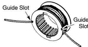
9. Insert the ends of the lines through exit holes in the sides of the cover.
