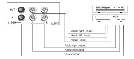
There is also an AV input on the front of your television. Use the Left Audio input (white terminal on the TV), if you are connecting equipment with mono sound. The MONO sound will be delivered by both left and right speakers.
