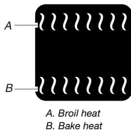
The CleanBake™ element is hidden under the floor of the oven, protected from spills and drips
